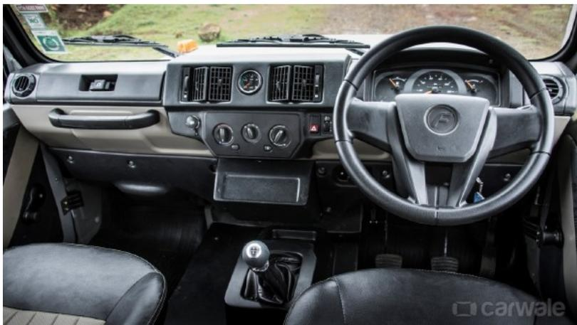
Unlike the Xplorer, the Xpedition is meant for the road and be a full-fledged family car. In that regard, it's pretty basic. Sure, you get power steering and an aircon, and a tiny glovebox. But, otherwise there's no real creature comfort to talk about. No power windows, no internal adjustment for the ORVMs, no rear wash and wipe and not a single cup or bottle holder either.
