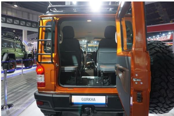
There is a step at the back for passengers to get in and out of the rear door comfortably. The toe-hook next to it means business, allowing for the Gurkha to tow another vehicle quite easily.
